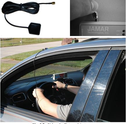
Fig. 2.7 - Using the External Antenna
