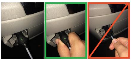
Fig. 2.6 - Proper Disconnection of Cigarette Lighter Adapter
