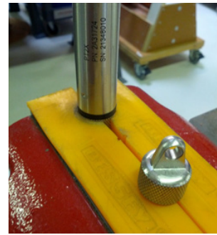
Cableless Sensor—gripping on knurled area
