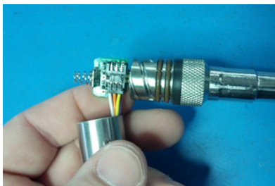
Connector connected properly
