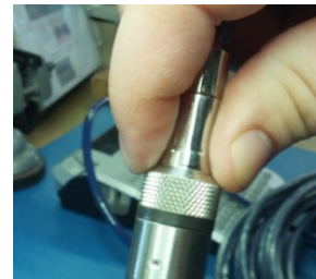
Properly completed—black ring uncompressed
